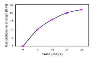
**Research results**: These specimens are tested by the machine compression testing after 7 days of concrete curing, 14 days of curing and 28 days of curing. The strength of concrete gradually increases with its age. Concrete is getting stronger day by day and after 28 days it is possible to identify its strength and strength grade.
