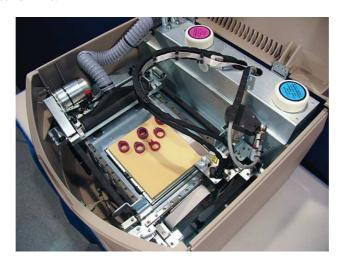
A master-model (a processed work piece) is used to make a «rubber»- an elastic mould consisting of two halves. A «rubber» is necessary to get wax copies of a master-model for a future jewel.
