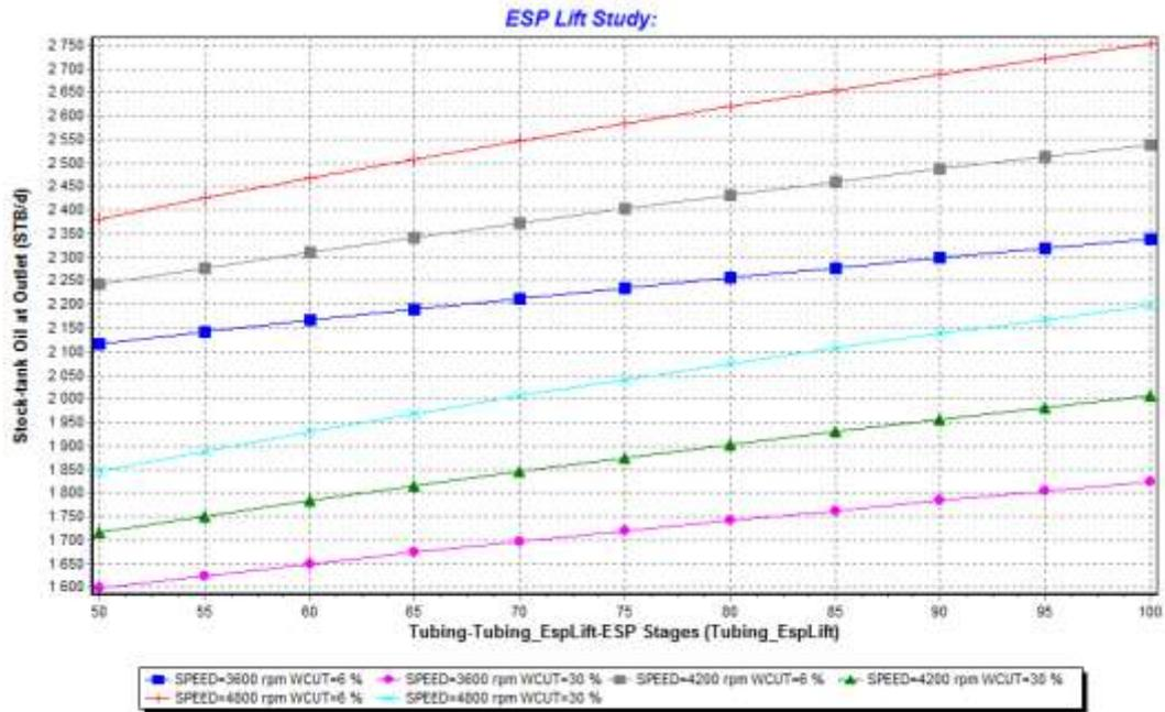
Figure 6 – The performance curve for ESP
