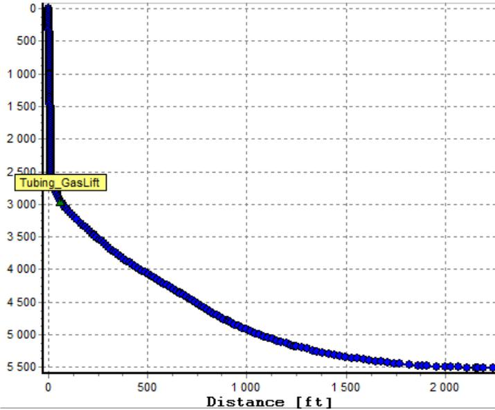
Figure 3 – The position of gas injection
